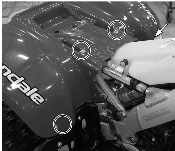
Rear fender bolts (3 of 4 visible in photo)
